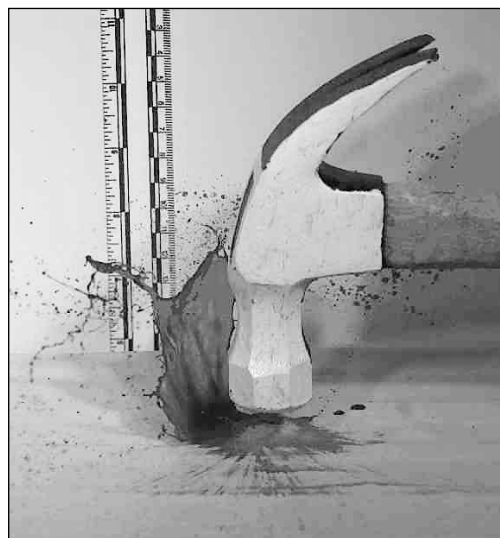
Active spatter created by the action of a hammer with dispersion of the fluid and central liquid lamella formation
