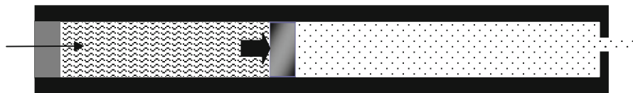
Fig. 2.5 Implantable cylindrical osmotic pump with piston. Water flows through semipermeable membrane at left into a chamber containing osmotic excipient ( curlies ), displacing piston, which in turn pushes drug formulation ( dots ) out through the orifice at right
